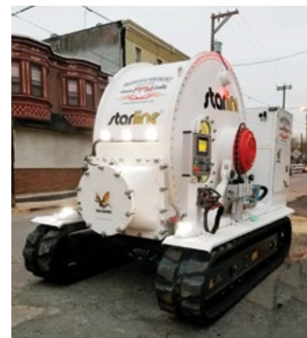
Super-sized drum for large diameter lining
