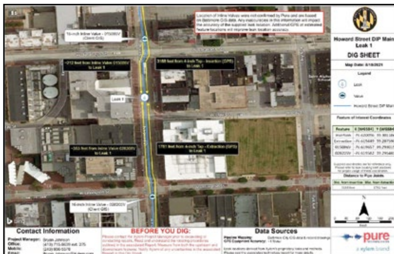
Figure 4: Dig Sheet showing location of Leak 1 under Howard Street
