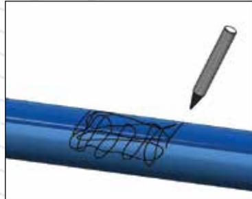
Mark the pipe surface to be scraped with a crisscross pattern
