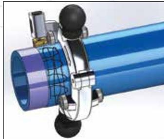
Scrape or peel the pipe to remove the surface layer and expose clean virgin pipe beneath
