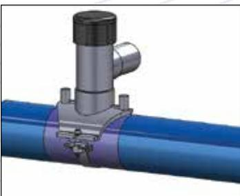
Clean surfaces with Isopropyl alcohol if necessary, avoid touching cleaned surfaces and clamp saddle to the scraped pipe using only the clamp provided or recommended by the fitting manufacturer
