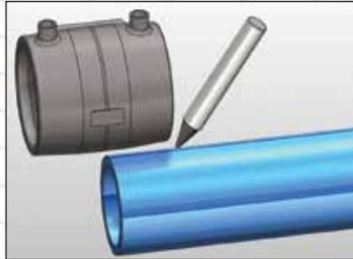
Measure and mark the stub ends on both pipe ends
