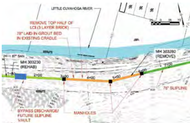
Figure 5 – Same Trench Replacement at Sag
