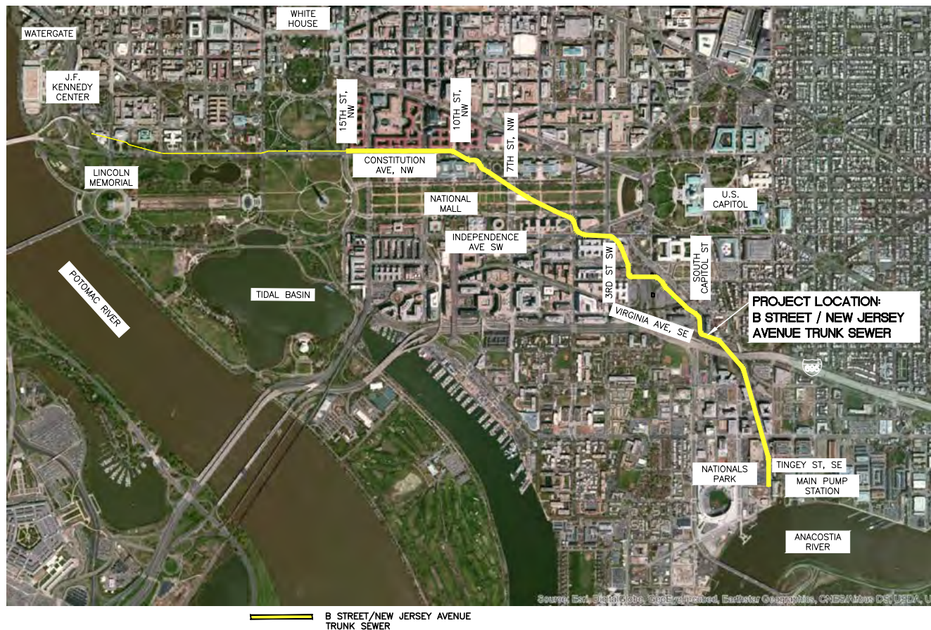
This historic unreinforced concrete sewer runs through the heart of the nation's Capital. The sewer extends approximately 22,700 linear feet and ranges in size from 6-foot-6-inch-diameter circular sections to an 18-foot-by-16-foot arched cross section.
