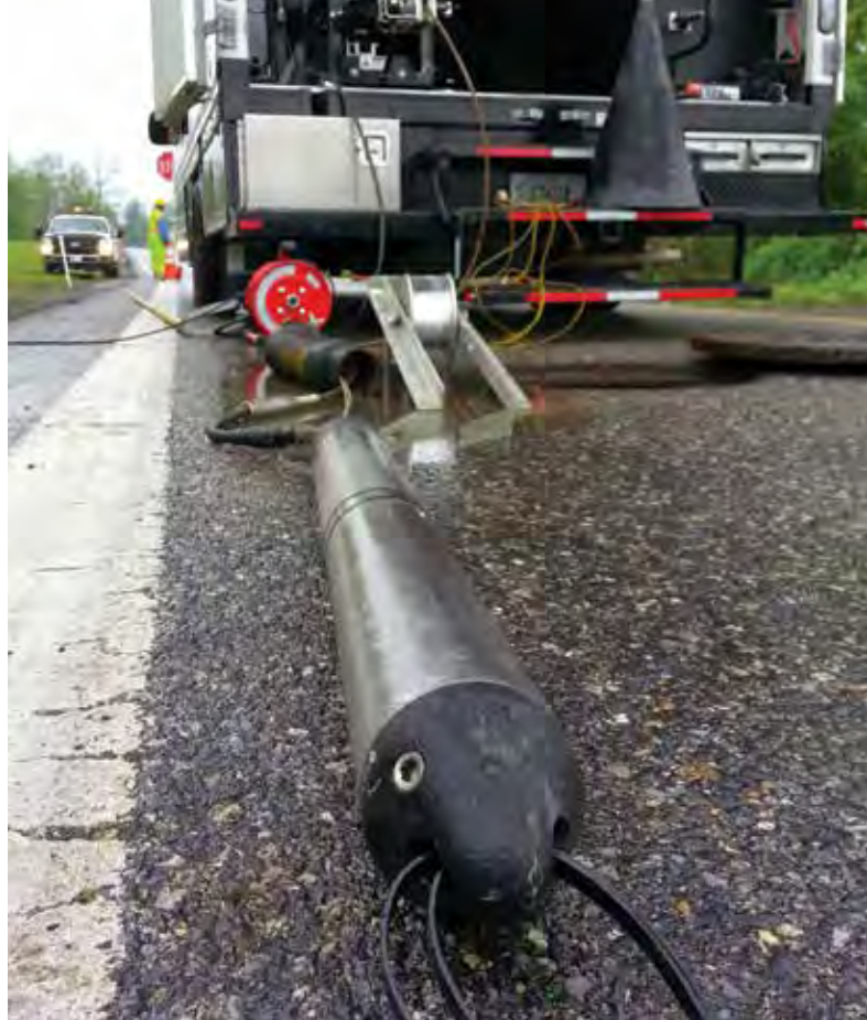
The Electro Scan ES 620 Probe, integrated into a standard CUES CCTV truck, gets prepped for the day's activities
