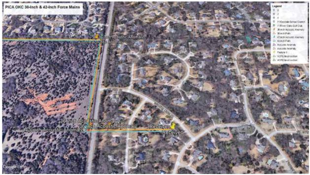
Figure 4. Zoom of the pipeline section of the 36-inch and 42-inch force mains with the acoustic anomalies. Based on the locations and confirmation of the air-pockets OKCWUT will perform external validations utilizing the PICA Bracelet Probe (Figure 2) to identify the wall loss in these areas and determine the RUL (Remaining Useful Life) of this critical asset
