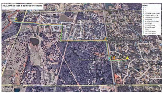
Figure 3. Identifies the inspection area of the twin force mains. The area located in the Green had been previously rehabilitated. The acoustic anomalies are identified with pins on each line
