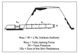
Figure 1: Free Body Diagram of the Forces acting on Pipe Jacking methods
