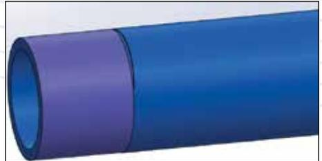
Inspect the scraped pipe surface thoroughly to ensure that all marks are removed and that only virgin pipe surface is exposed
